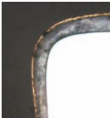
Cross-section of a drug coated stent, gold coated to protect the drug during preparation, 500x.
