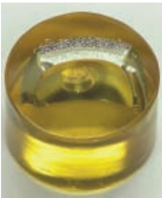
Acetabular Cup mounted in EpoHeat® Epoxy.
