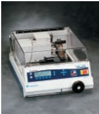
IsoMet® 5000 Linear Precision Saw. Options include a Bone Chuck, Glass Slide Chuck and Irregular Specimen Chuck.
