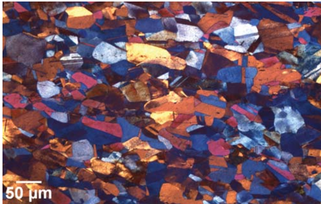
Figure 4: Microstructure of wrought, annealed tough-pitch copper; top: etched with equal parts ammonium hydroxide and hydrogen peroxide (3% conc); bottom: Beraha's PbS tint etch, polarized light plus sensitive tint illumination.
