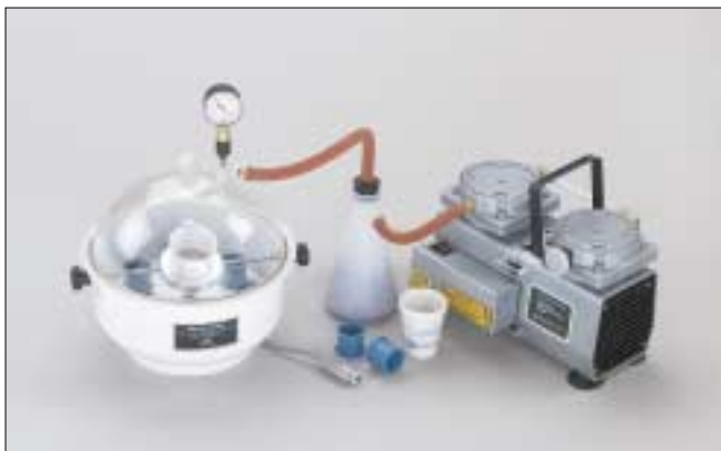
Figure 4. VACUUM IMPREGNATION device used to fill pores in bones with epoxy. Several specimens can be impregnated simultaneously.
