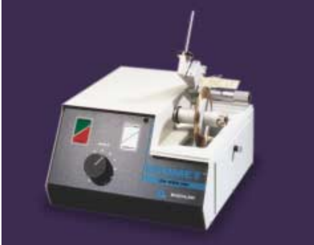
Figure 2. ISOMET® Low Speed Saw used for sectioning biomedical materials
