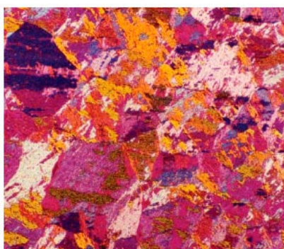
Fig. 5. Low-carbon martensite in Carpenter Technology's AerMet 100 ultrahigh-strength steel (Fe-0.23% C-13.5% Co-11.1% Ni-3.1% Cr-1.2% Mo) heat treated (1093°C, AC, age at 675°C for 6 h, AC) to coarsen the grain size and etched with 10% sodium metabisulfite (100x)
