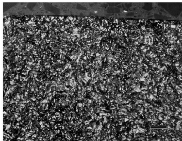
Fig. 8. Surface of a carburized 8720 alloy-steel railroad-cone bearing etched with nital plus 1% zephiran chloride. Image analysis yielded 13.3% retained austenite vs 25.4% by XRD (1000x).
