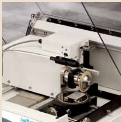
The 11-2694-115 Precision Table for sectioning thin materials rotates 180° in 1° increments to facilitate sectioning along a line of features on a die.
