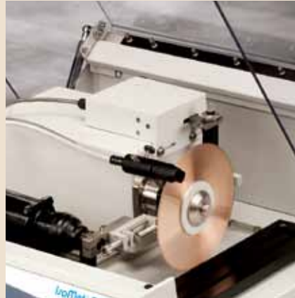
Stainless steel fastener vise 11-2687 allows longitudinal sectioning for examination of thread machining and heat treat.
