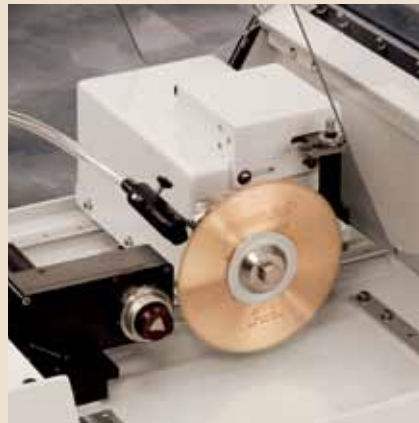
Accessory rotating vise 11-2695 with Minimal Area of Contact Cutting (MACC) reduces cut time, doubles sectioning capacity and maximizes samples cooling.
