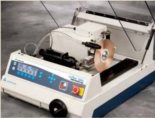
The IsoMet's feature a spacious interior, versatile sample fixturing and easy sample retrieval. Manual Blade Positioning Handle provides quick setup. The IsoMet's precision is a result in the superior mechanical design, precision linear bearings and vibration dampening aluminum casting. Removal X and Y-axis T-Slot beds allow sample positioning on either axis.
