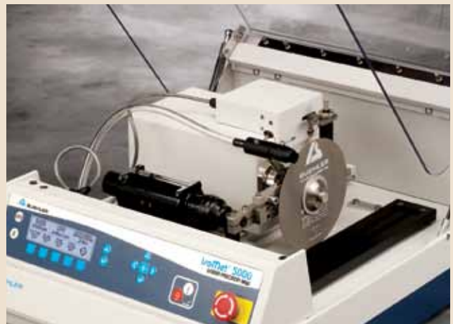
Since adequate coolant volume and positioning is critical for good cutting, the IsoMets provide a full 0.7gal/min (3ℓ/min) presented to both sides of the blade. The coolant tracks with the blade for long cuts.
