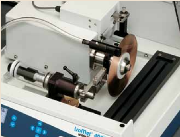
The IsoMet® 4000 has a manual 1µm sample positioning via a precision micrometer. The blade advances automatically and is retracted manually.
