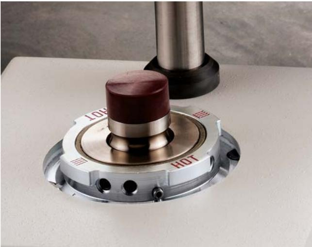
Hot compression mounting produces a reliable and consistent specimen mount.
