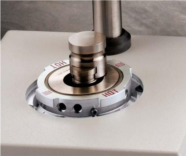
Changing mold assemblies is quick and easy due to the lower ram dovetail connection design.
