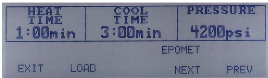
On the SimpliMet 3000, use the Load, Next and Previous functions to save up to 25 user defined methods and to access the four Buehler methods.
