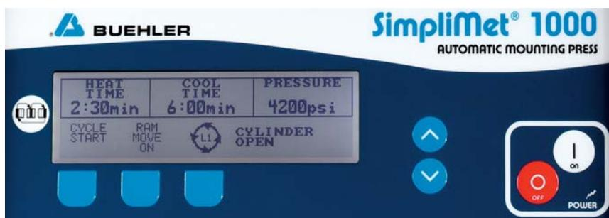
The SimpliMet 1000 (top) and SimpliMet 3000 (bottom) feature a Liquid Crystal Display (LCD) with easy-to-use touch panel controls. Simply scroll to the desired parameter and adjust with the up/down arrow keys.
