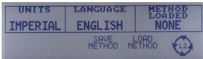
The second screen controls Units of Measure and Language. On the SimpliMet 3000, the loading and saving methods are also displayed for operator convenience. "None" is displayed under method loaded when the operator changes the parameters to differ from a loaded method.
