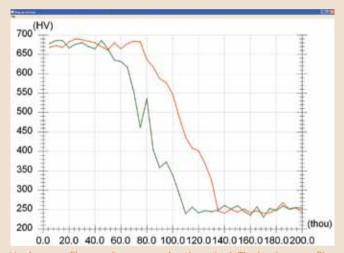
Hardness profiles may be measured and graphed. The hardness profile shown above is typical for case hardened specimens. As hardness is measured from the surface to the inner bulk of the material the hardness value reduces dramatically
