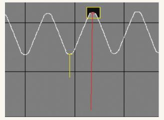
Once the outline of a specimen is traced it can be viewed in the Stage Overview window. This offers precision control of stage positioning to increases efficiency and productivity when identifying suitable measurement locations. The yellow and red lines in the window represent locations where multi-indent hardness profiles will be measured.
