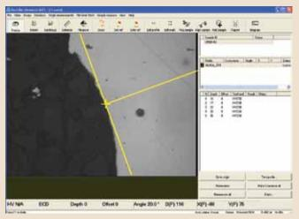
The OmniMet® MHT Graphical User Interface (GUI) is designed for ease-of-use - with good workflow using a few simple-to-understand icons to run the hardness test. Here the GUI is shown with the alignment tool for setting the direction of a profile perpendicular to the specimen surface.
