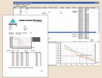
OmniMet® MHT has an integrated database that archives all measurements. Data may be retrieved at any time, reviewed, or sent to automatically generated reports as shown above. Report templates are completely customizable by the operator to suit the measurements being undertaken.
