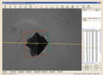
OmniMet® MHT's indent measurement algorithms detect indents and automatically measure the Vickers or Knoop hardness of the specimen. Additionally, conversions into Rockwell B or C scales is also supported. Measurement of a Vickers indent is depicted above.
